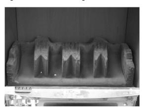
b) Place the left hand front coal rail moulding onto the front ceramic rail support and locating pins as shown below in Fig. 4
