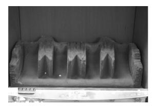
b) Place the left hand front coal rail moulding onto the front ceramic rail support and locating pins as shown below in Fig. 17
