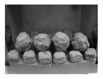
e) Select three of the small coals and fit onto the ribs of the fuel-bed base. See fig. 7 below
