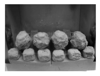
e) Select three of the small coals and fit onto the ribs of the fuel-bed base. See fig. 20 below
