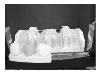
c) Place the right hand front pebble rail moulding onto the front ceramic rail support and locating pins as shown below in Fig. 26
