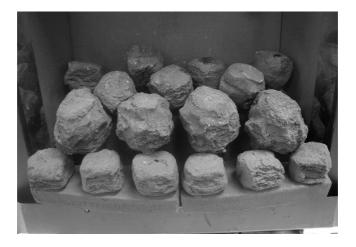
g) Ensure the coals sizes are correctly positioned as shown in Fig. 9 below. "L" denotes "large" coals and "S" denotes small coals. If any coals are missing, please contact your retailer. Do not proceed with the installation.
